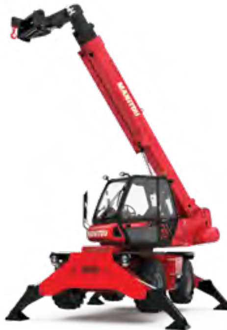
Rotation on lowered stabilisers with 1500 kg jib
