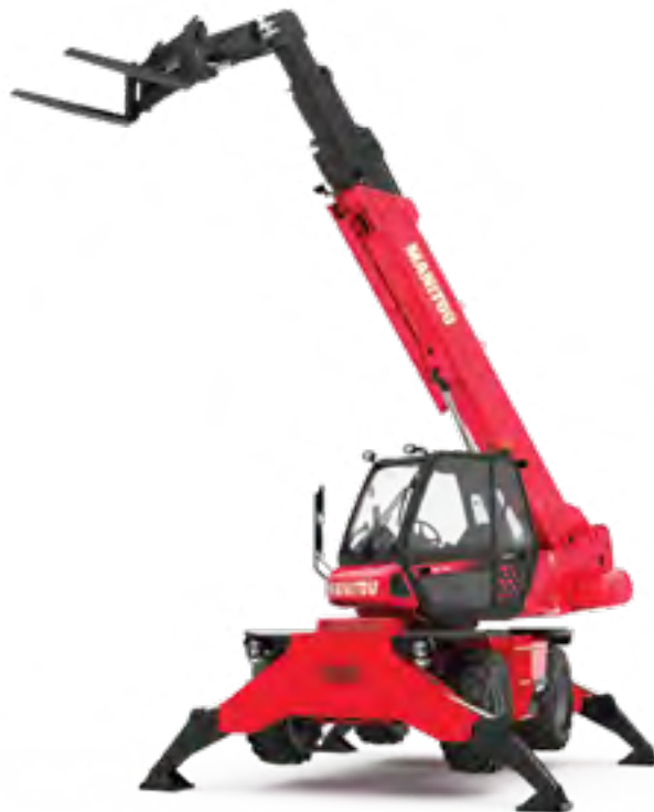
Rotation on lowered stabilisers with 1500 kg jib
