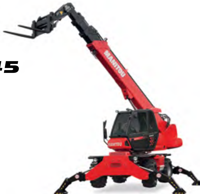
Rotation on lowered stabilisers with 1500 kg jib
