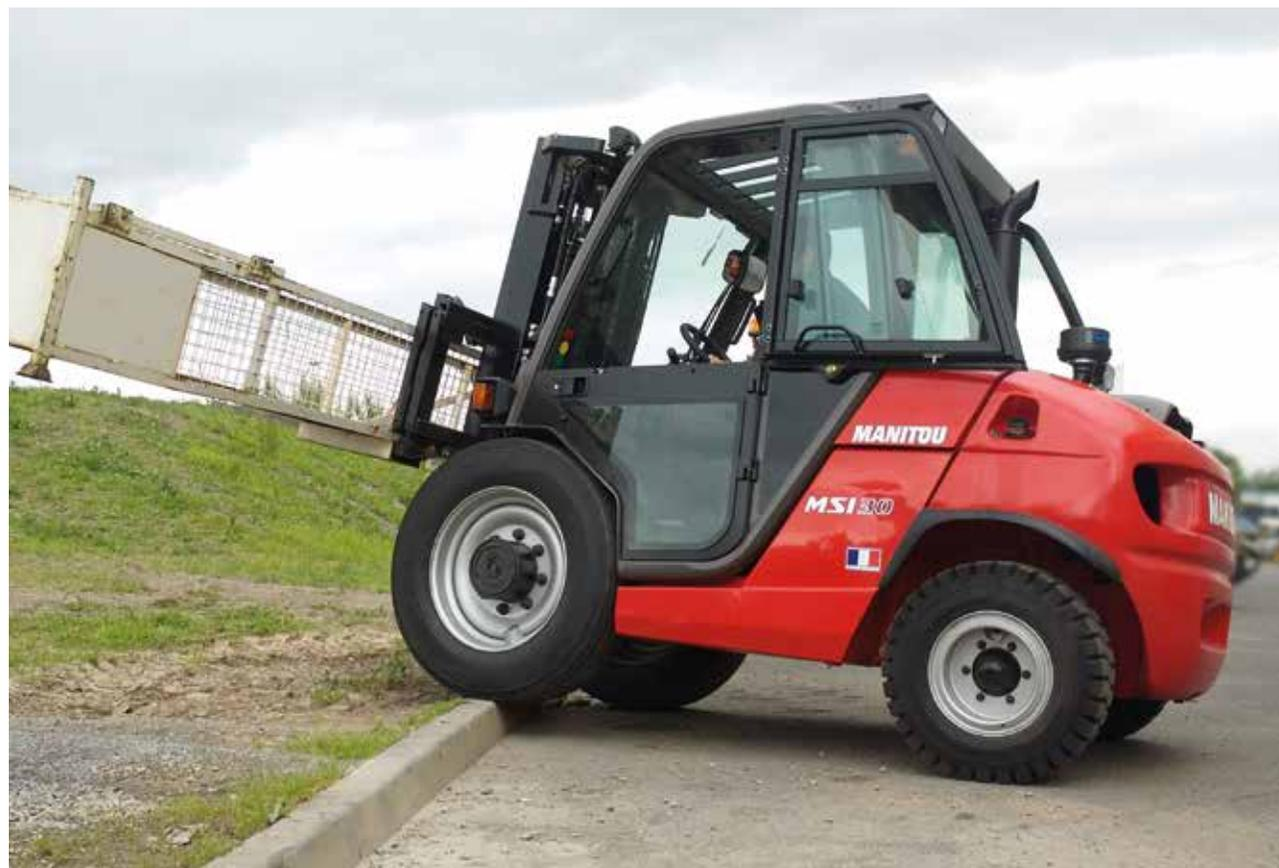
Work easily in confined spaces. With their compact dimensions and a very tight turning radius (thanks to the steering axle with built-in cylinder), MSIs provide exceptional mobility.
