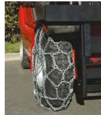
The chassis design allows chains to be fitted and provides optimum traction under extreme conditions.
