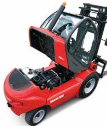
The electro-hydraulic tilting of MH cabins ensure quick access to mechanical components for easy servicing.
